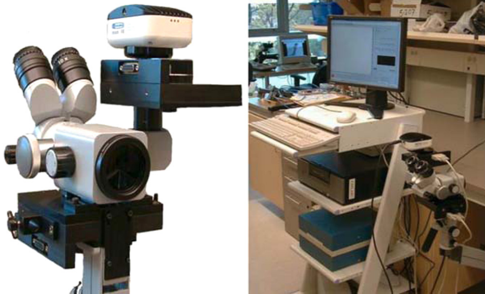
Figure 3. The multispectral digital colposcope (MDC). The left panel shows the imaging component of the MDC; the right panel shows the associated computer equipment required to operate the device and store imaging data.
