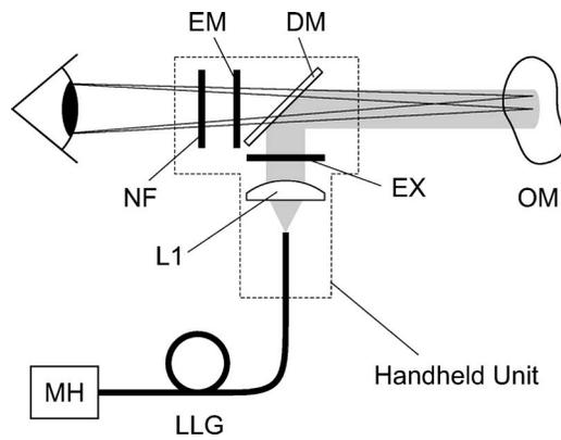
**Fig. 1** Schematic diagram of device for direct FV of oral mucosa: metal-halide light source (MH), liquid light guide (LLG), collimator lens (L1), excitation filter (EX), dichroic mirror (DM), oral mucosa (OM), emission filter (EM), and notch filter (NF).
